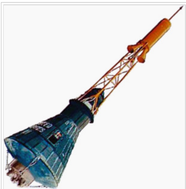
The Mercury Capsule design (shown with escape tower) originally used a radiatively cooled TPS but was later converted to an ablative TPS
