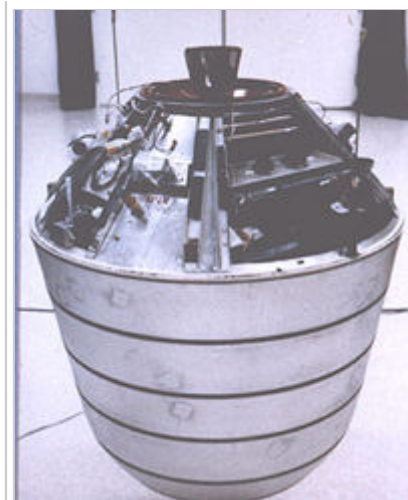
"Discoverer" type reconnaissance satellite film Recovery Vehicle (RV)
